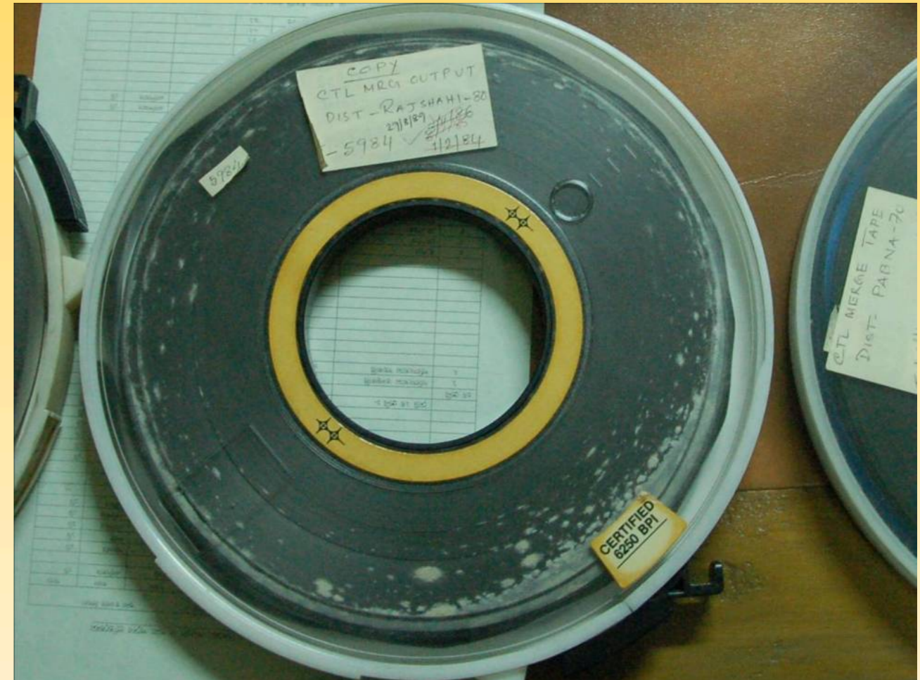
1973 census tape #1: manual spacing required to recover data
