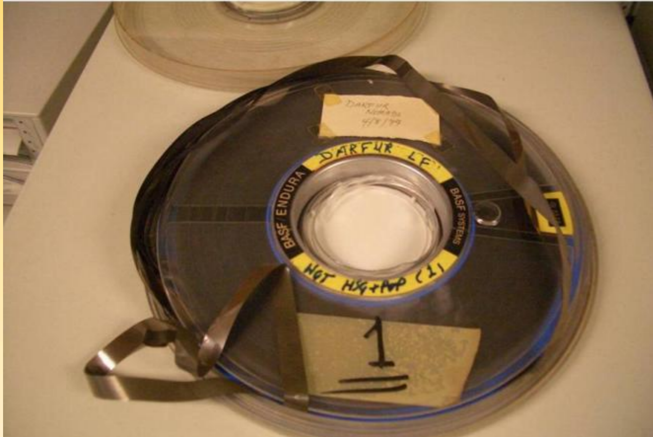
1973 census tape #1: manual spacing required to recover data
